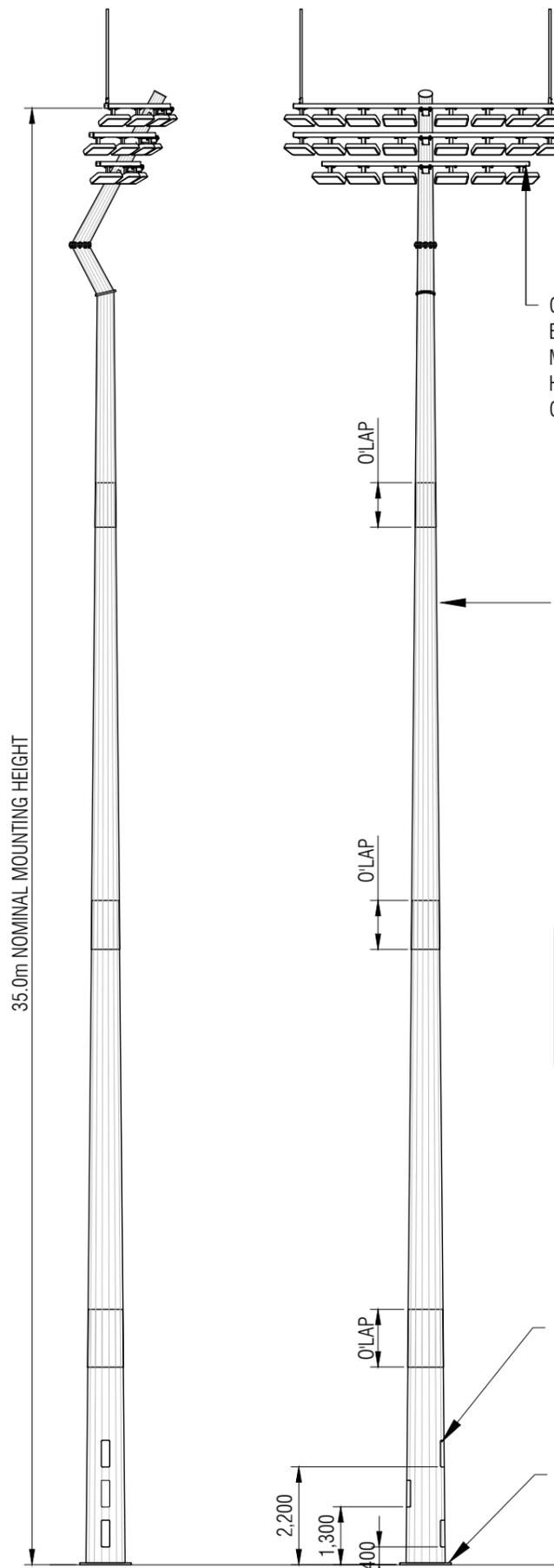
GM POLES MANUFACTURED UPPER AND MIDDLE CURVED CROSSARM TO SUIT 8x VAILO ZENITH GEN V 1500w LIGHT FITTINGS MOUNTED UNDERSLUNG AT UP TO 40° LENS TILT TO HORIZONTAL. NO ALLOWANCE FOR EXTERNAL GLARE CONTROL DEVICES. REFER DETAIL "B".
